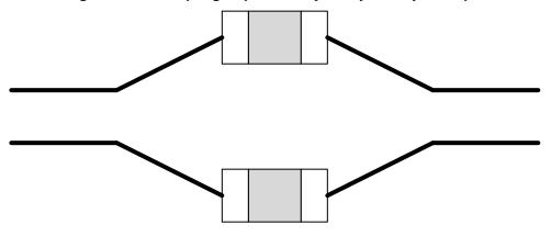
**NOTE:** Adding test points to the high-speed traces can cause impedance discontinuity which negatively impacts signal performance. If test points are used, they should be placed in series and symmetrically. They must not be placed in a manner that causes a stub on the transmission line.
