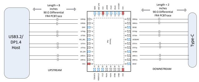
Using the given trace lengths and data rate in this example, the method to select the equalization values for Upstream and Downtream EQ is to select the closest EQ gain value available to match the trace loss as follows.
