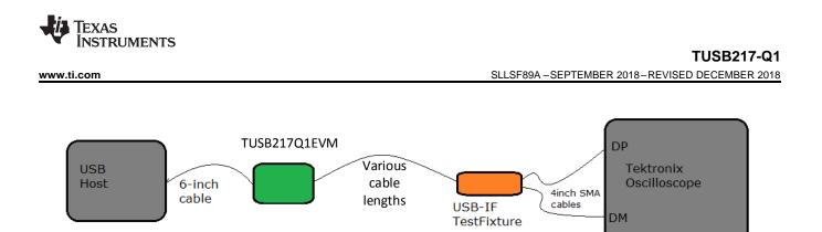
Figure 21. Near end eye measurement set up with post-channel cable
