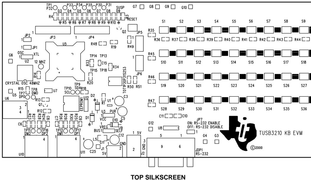
Figure 1–4. TUSB3210 Keyboard Evaluation Board Rev. 3—Silkscreen
