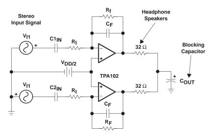
Figure 3. TPA102 Audio Amplifier-Single Capacitor Configuration
