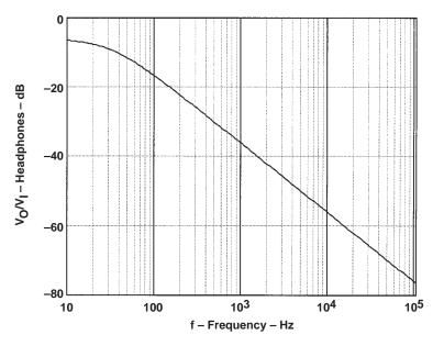
Figure 5. Crosstalk vs Frequency for a 32-Ω-Load and a Single 330-µF-Coupling Capacitor
