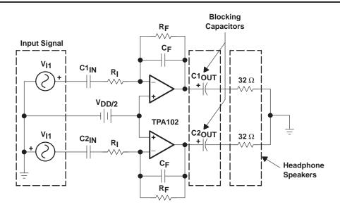
Figure 2. TPA102 Audio Amplifier-Dual Capacitor Configuration
