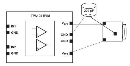
Figure 7. Lab Setup for the TPA102 EVM
