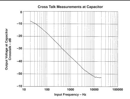
Figure 8. Crosstalk Measurement of Single Capacitor Configuration
