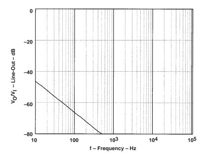
Figure 6. Crosstalk vs Frequency for a 10-k $\Omega$ -Load and a Single 330- $\mu$ F-Coupling Capacitor
