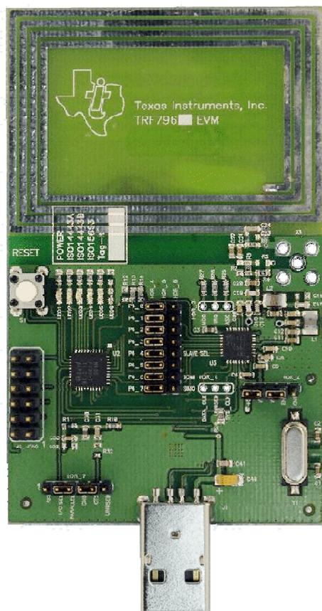
**Figure 1. The TRF7960 Evaluation Module**
