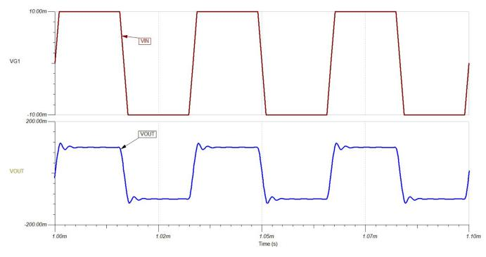
Figure 11. Transient Response - Active Feedback with Secondary Compensation
