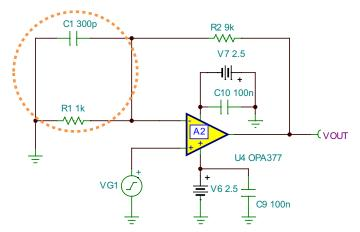
Figure 1. Phase Compensation Using RC Circuit
