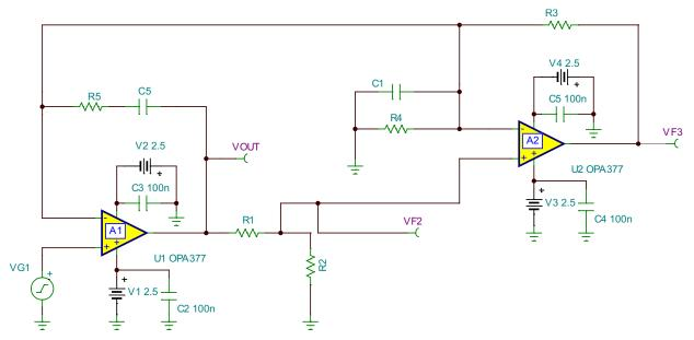
Figure 9. Active Feedback with Secondary Compensation
