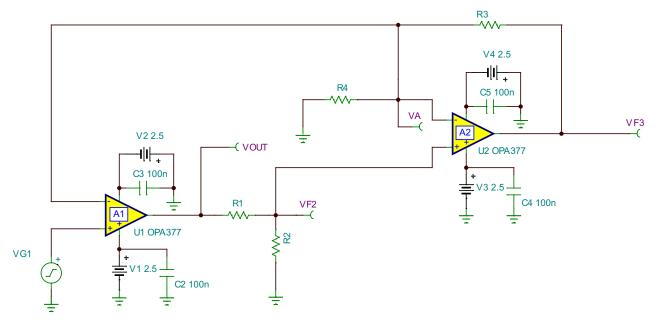
Figure 3. Active Feedback Compensation Scheme
