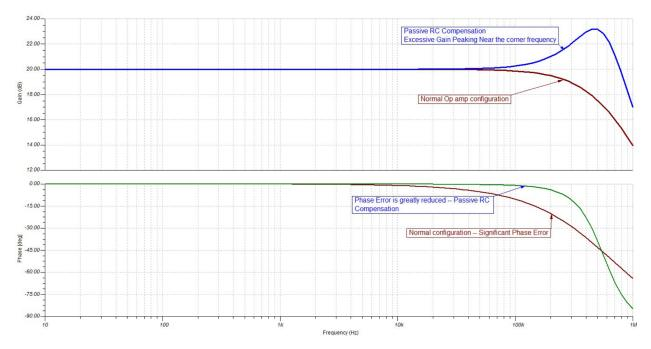
Figure 2. Amplitude and Phase Response of the Passive RC Method
