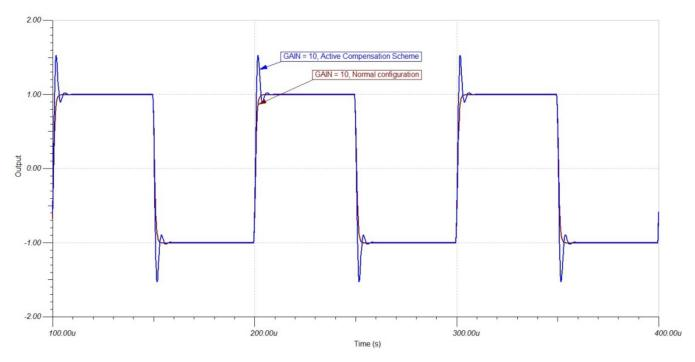
Figure 7. Transient Response of the System with Gain 10
