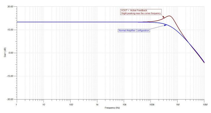
Figure 6. Amplitude Response of Normal and Active Feedback Compensation Scheme
