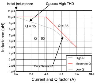
Figure 5. Inductance Versus Current and Q Factor
