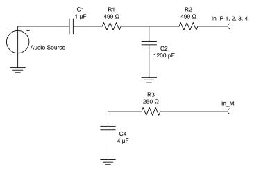
Figure 1. TAS5414C Input Circuit
