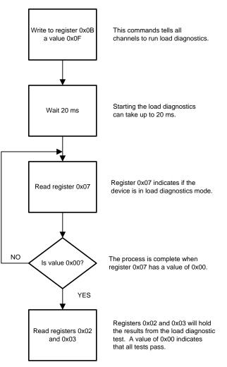
Figure 13. Load Diagnostics, Four Channels
