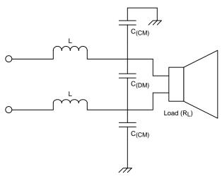
Figure 4. Typical Output Demodulation Filter
