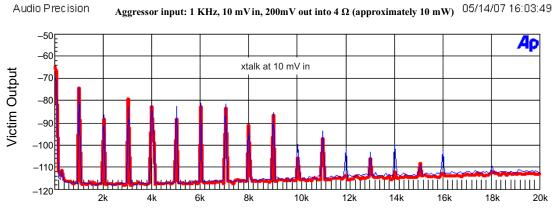
Figure 8. Channel 1  $\rightarrow$  Channel 3 Harmonic Crosstalk With Default Switching Phase Settings
