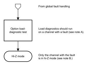
Figure 15. Channel Fault Handling
