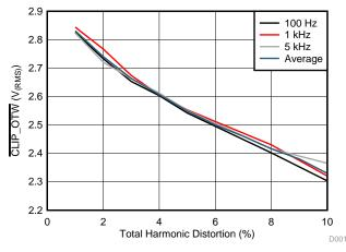
Figure 6. <u>CLIP</u>OTW Pin Voltage Versus % of THD
