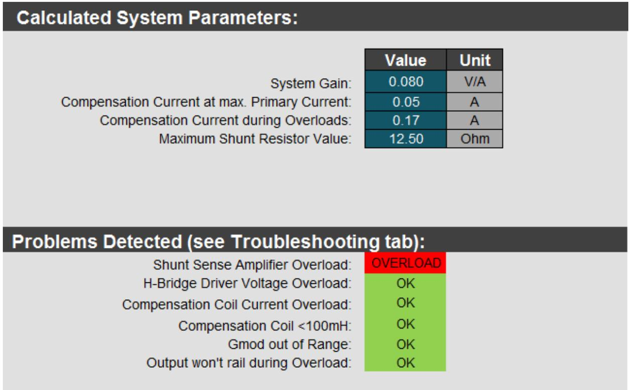
**Figure 2. Calculated Outputs**
