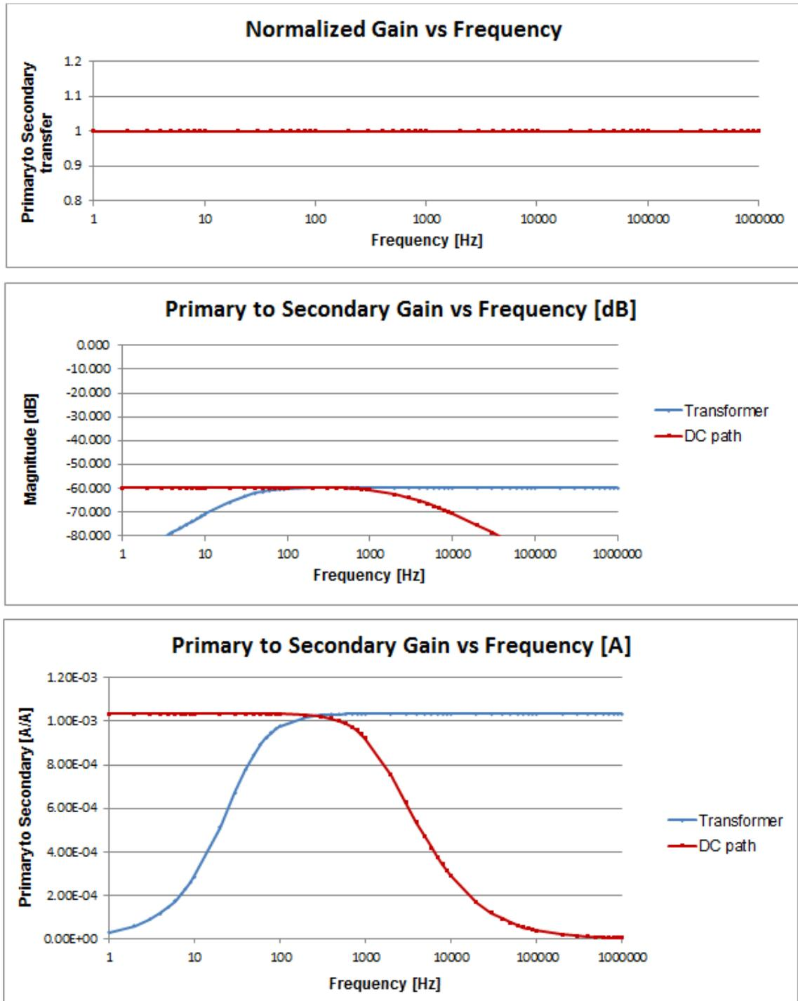
Figure 5. Closed Loop Gain vs. Frequency Response
