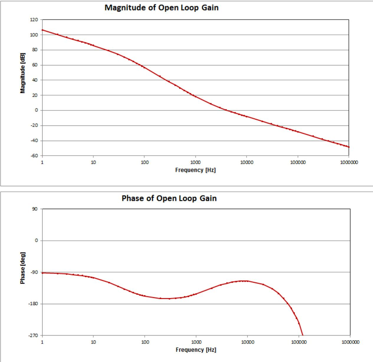
**Figure 4. Open Loop Gain and Phase Response**
