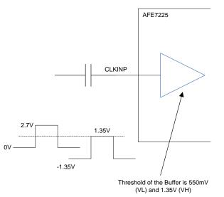
Figure 2. Single Ended Clock Buffer in AFE7225
