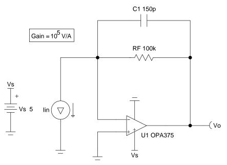
For the circuit in Figure 15, the gain can be calculated using the following equation:
