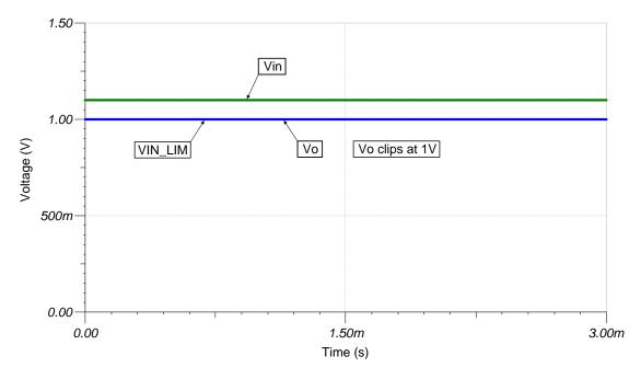
When designing a buffer circuit, RRI amplifiers are not required as long as the following equation is satisfied.
