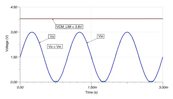
Figure 2. Transient simulation for AC buffer circuit example 1
