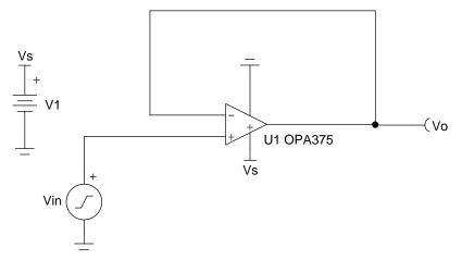
Solving Equation 2 for the OPA375 using  $V_s = 5 V$  yields Equation 3. This inequality must be true in order to avoid clipping or other non-linear behavior.
