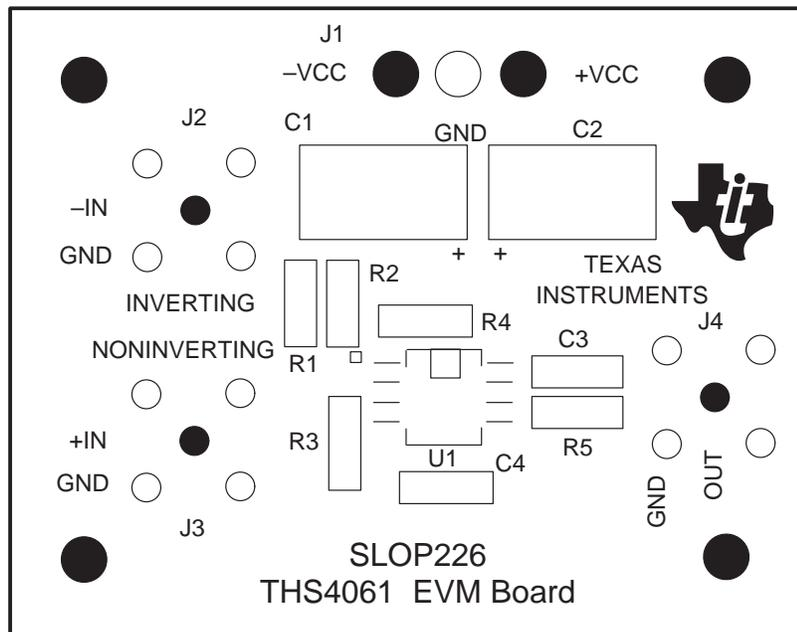
Figure 2–2. THS4061 EVM PC Board Layout – Component Side
