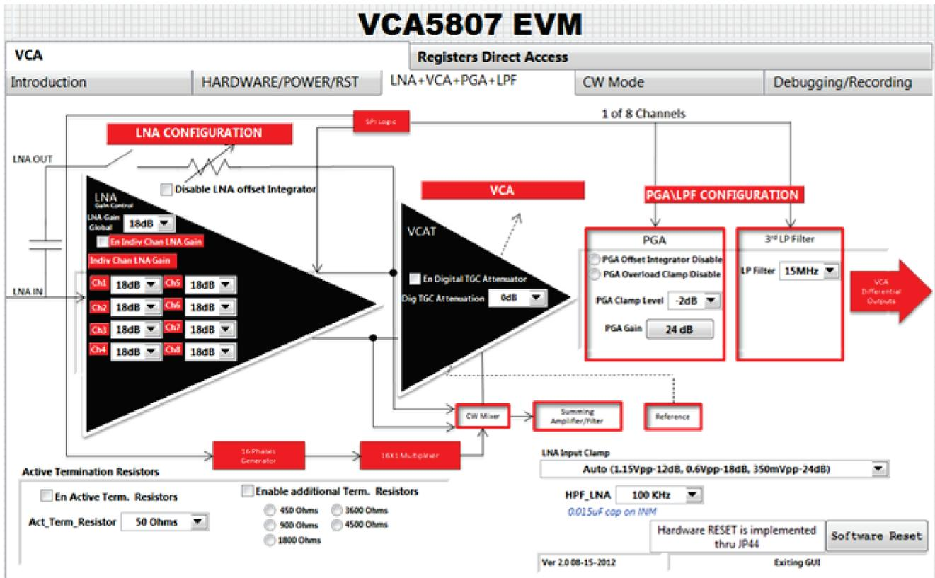
Figure 4. VCA LNA+VCA+PGA+LPF Tab of the VCA5807EVM GUI
