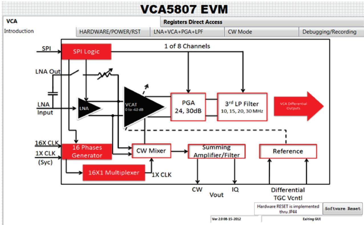
Figure 2. Introduction Tab of the VCA5807EVM GUI
