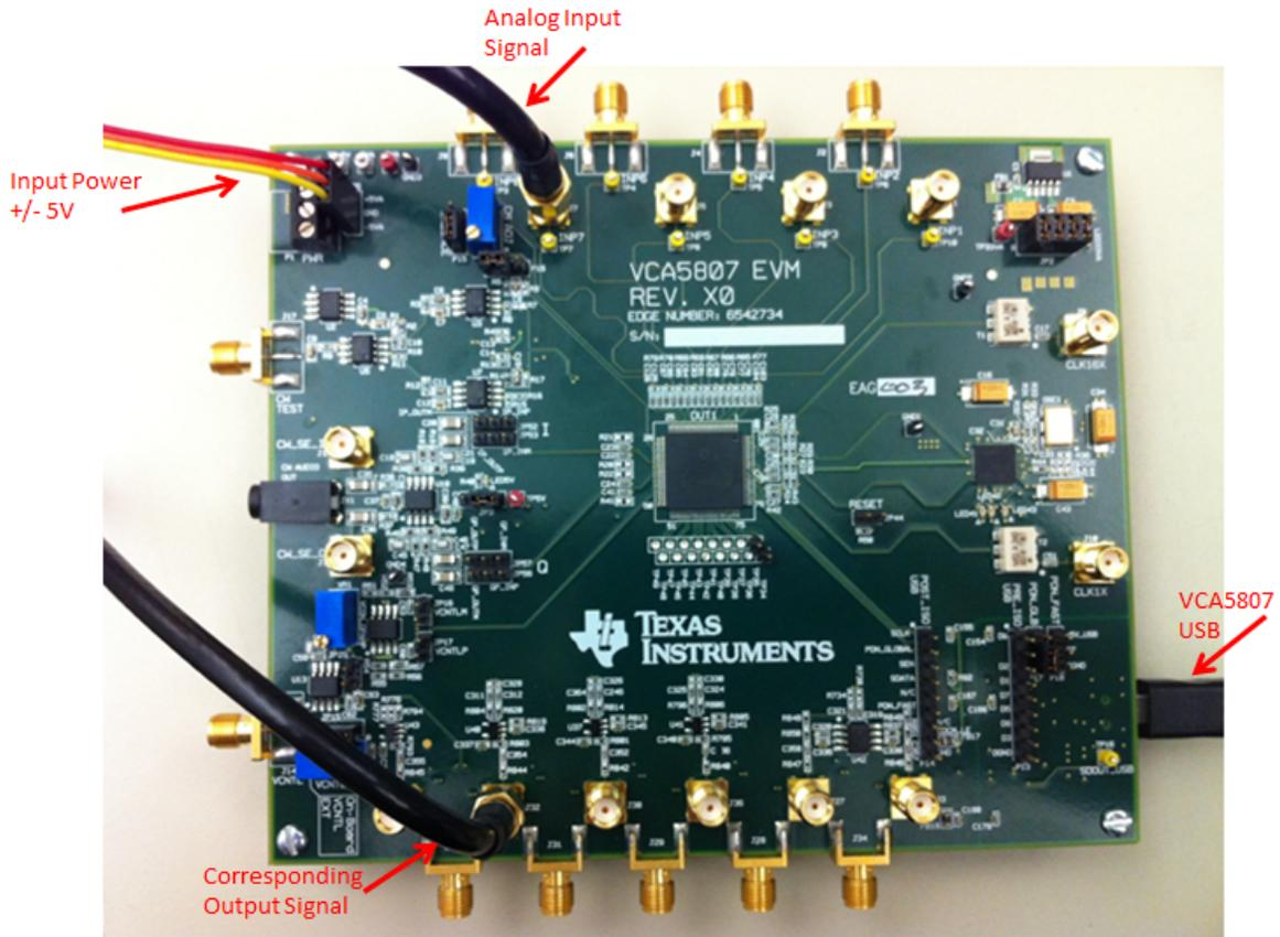
Figure 7. HW Setup
