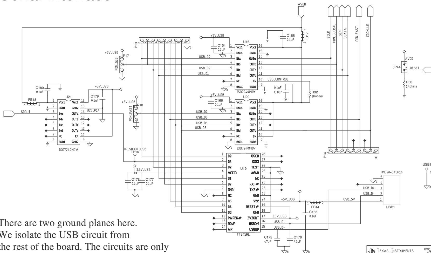
There are two ground planes here. We isolate the USB circuit from the rest of the board. The circuits are only coupled through the opto-isolators.
