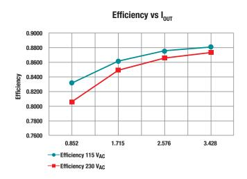
Figure 5. Efficiency vs.  $I_{OUT}$ ,  $V_{IN}$  115 VAC and 230 VAC
