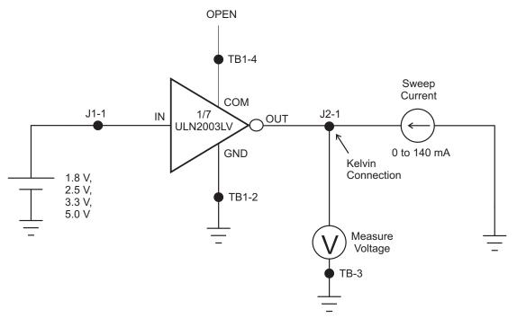
Figure 9. VOL Schematic
