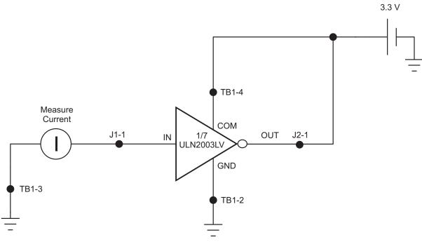
Figure 8. II(off) Schematic
