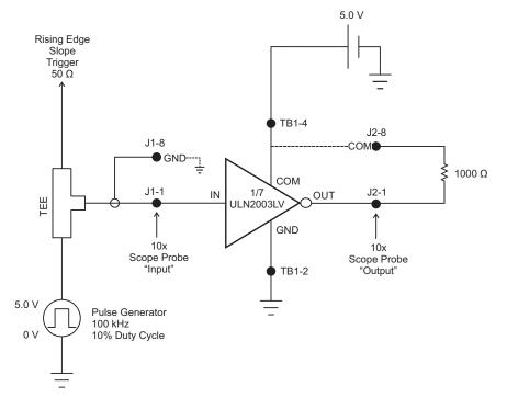
Figure 17. T<sub>PHL</sub> Schematic
