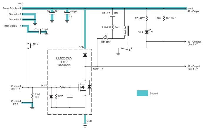
Figure 3. Single Channel Schematic
