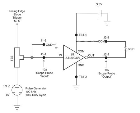
Figure 13. T<sub>PHL</sub> Schematic
