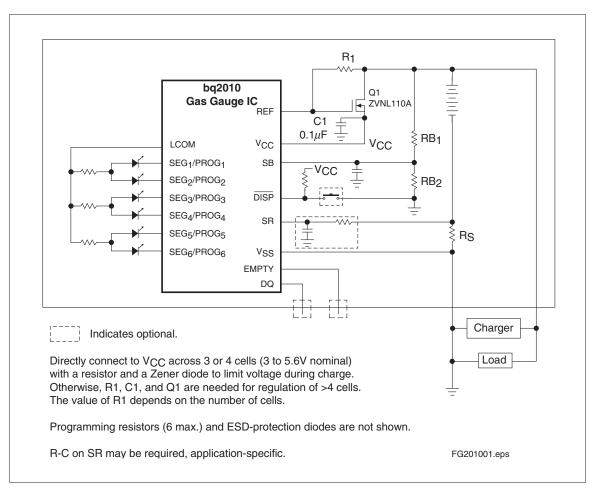
Figure 1. bq2010 Application Diagram—LED Display
