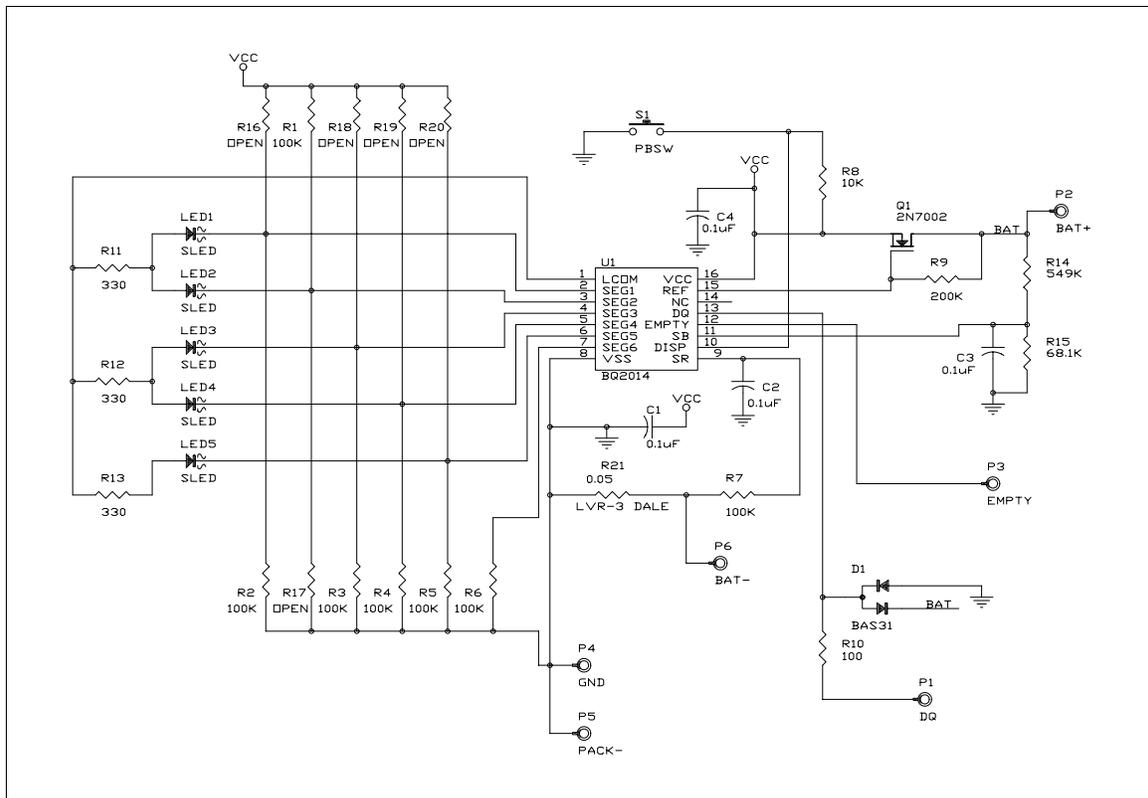
Figure 3. bq2014 NiMH Battery Capacity Monitoring System
