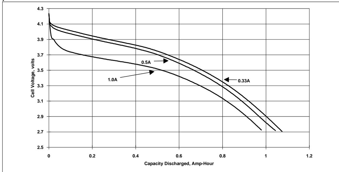
Figure 1. Li-Ion Battery Discharge Curve (Coke Electrodes)
