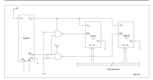
Using the bq4845 for a Low-Cost RTC/NVSRAM Subsystem
