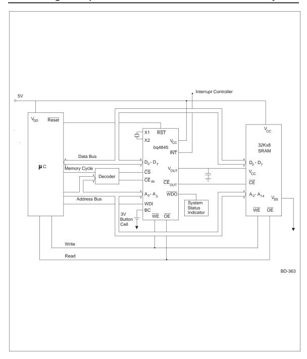
Using the bq4845 for a Low-Cost RTC/NVSRAM Subsystem
