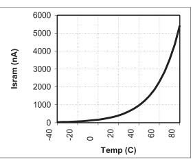
Figure 5. Typical L-LSRAM Data-Retention Current at V<sub>CC</sub> = 3V
