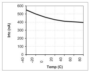
Figure 4. bq4845 Data-Retention Current at V<sub>BC</sub> = 3V
