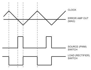
Figure 4. Circuit Waveforms (Switching Frequency)
