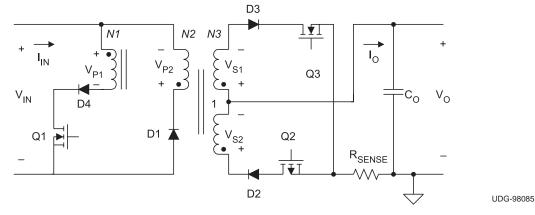
Figure 2. Four-quadrant Flyback Converter Topology
