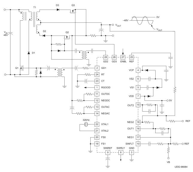
Figure 12. Alternative Implementation — N-channel Q2
