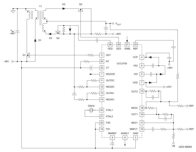
Figure 11. Non-isolated Ring Generator Implementation
