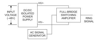
Figure 1b. Conventional Ring Generation Using Full-Bridge Amplifier
