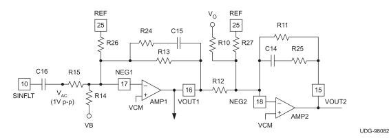
Figure 8. Summing Amplifier and Error Amplifier Configuration
