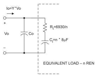
Figure 5. Equivalent Load of n Phones as Seen by the 4-Quadrant Ring Generator
