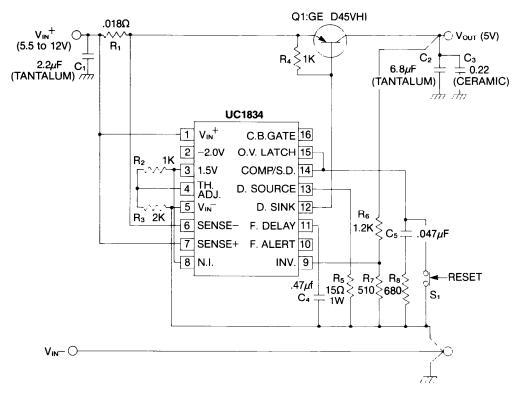
Figure 17. 0.5V Input-Output Differential 5A Positive Regulator
