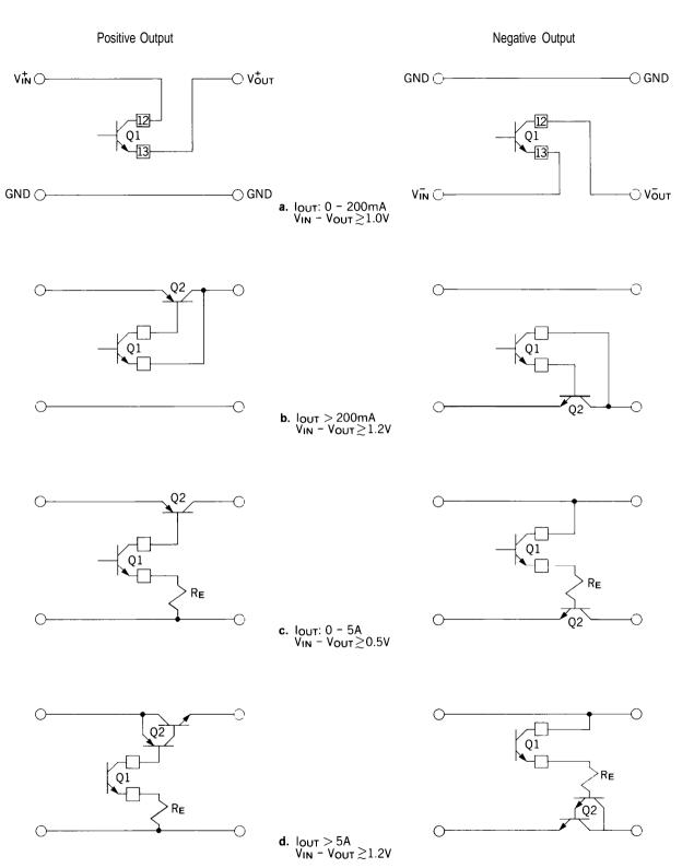
Figure 3. Pass Transistor Configurations
