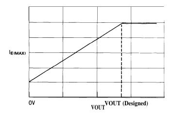
Figure 13. Foldback Current Limiting Characteristic
