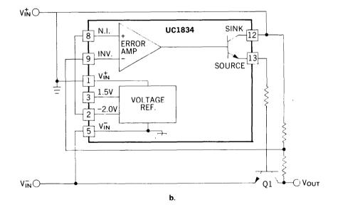
Figure 1. Basic Elements of (a.) Positive and (b.) Negative Regulators implemented with a UC1834
