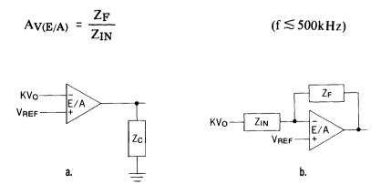
Figure 21. E/A Compensation (a.) Without and (b.) With Local Feedback
