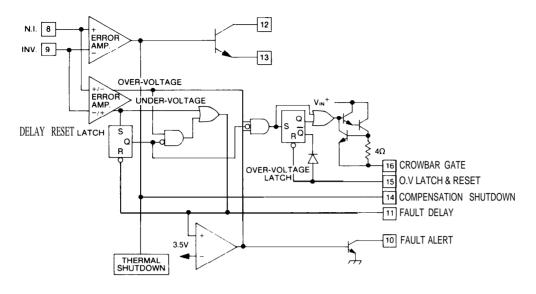
Figure 14. Fault Circuitry
