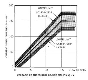
Figure 6. Guaranteed Tolerances on C/S Threshold Adjustment
