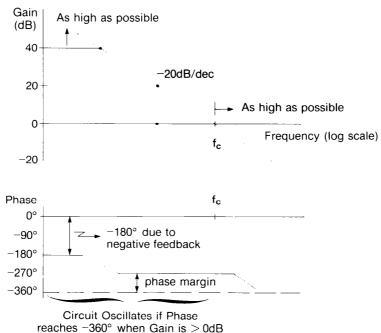
Figure 15. Desired Closed-Loop Response
