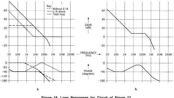
Figure 18. Loop Responses for Circuit of Figure 17 a. Voltage Loop b. Current Loop
