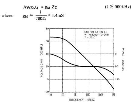
Figure 20. Error Amplifier Gain and Phase Frequency Response
