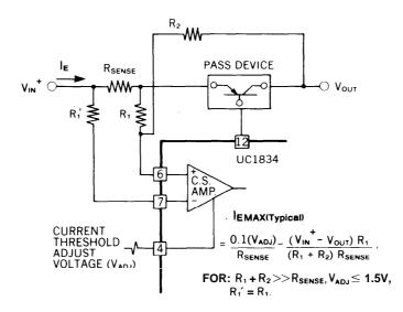
Figure 11. Foldback Current Limiting - Responds to Changes in VIN or VOUT
