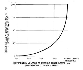
Figure 9. Current Limiting Knee Characteristic
