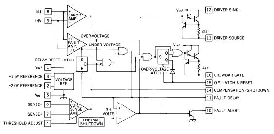
Figure 2. UC1834 Block Diagram
