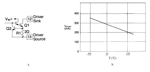
Figure 4 a. Driver Current Limiting Circuit b. Resulting Maximum Current vs Temperature
