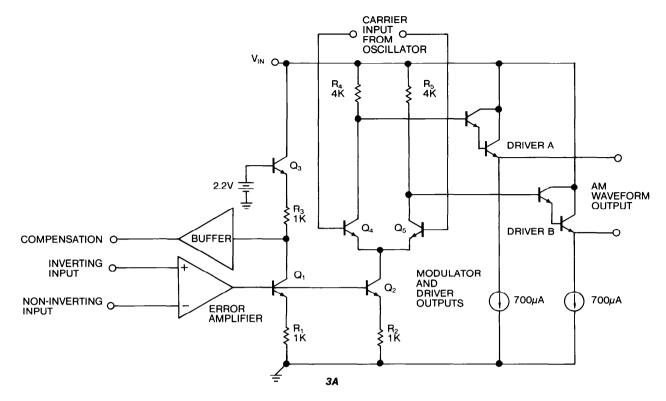
FIGURE 3: The Compensation Output on the UC7907 can be used to Accurately Control the AM Waveform Output.
