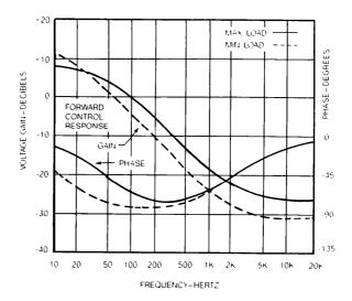
FIGURE 10: Closing the Feedback Loop is Preceeded by the Characterization of the Converter's Forward Small Signal Transfer Function.
