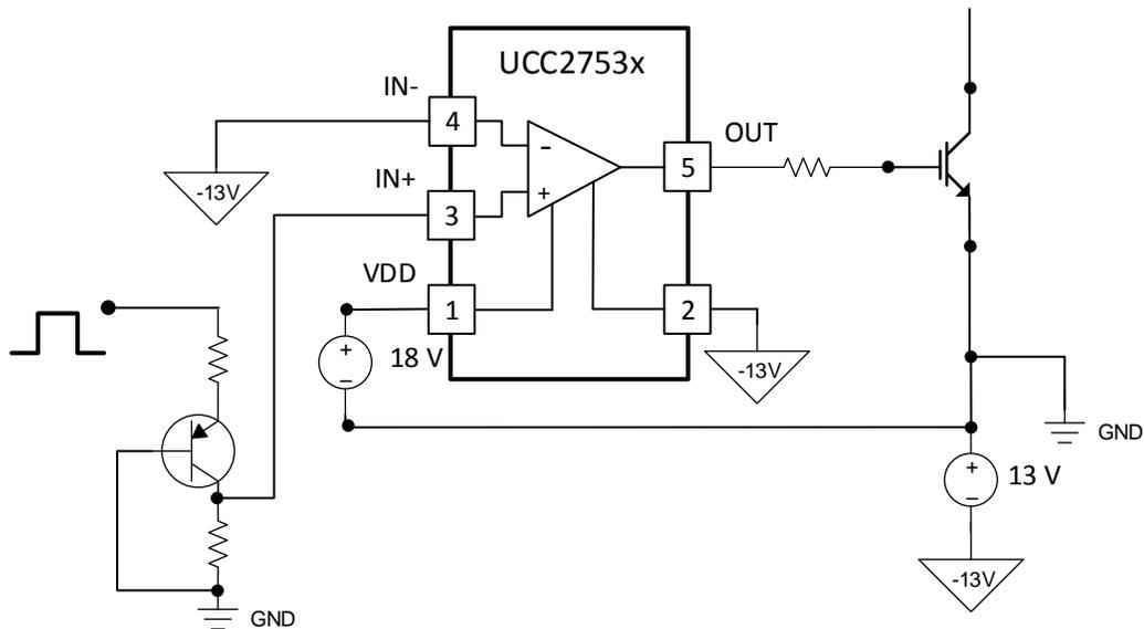
Figure 2. IGBT Bipolar Supply with Level Shifter
