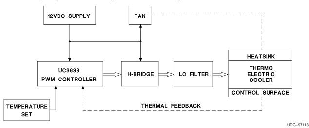
Figure 1. Temperature Controller Block Diagram
