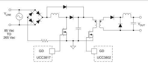
Figure 1. Two-Stage Power System
