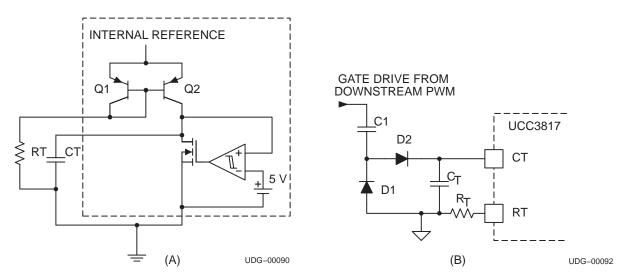
Figure 2. Internal Oscillator for a PFC Controller (A) and Synchronization Circuitry (B)
