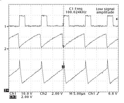
Figure 5. UCC3802 Oscillator Waveform with Synchronization
