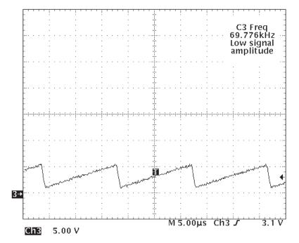
Figure 4. UCC3817 Oscillator Waveform Without Synchronization
