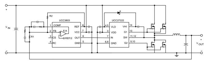
Figure 1. Low-Voltage Synchronous Buck Feedback Solution
