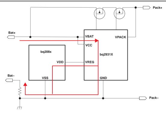
Figure 2. Measuring Board Offset With Power on Bat+ and Bat– Introduces Error From IC Operation Current
