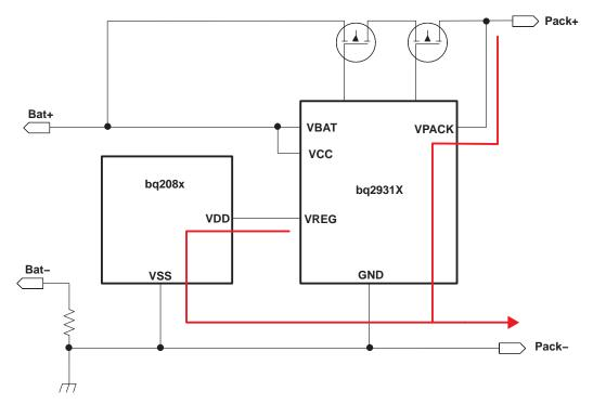
Figure 3. Powering ICs From Pack+ and Pack– Allows the IC Current to Bypass the Sense Resistor
