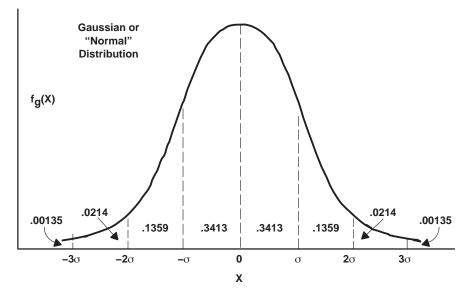
Figure 4. Gaussian Distribution Function
