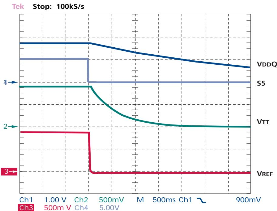
Note: After the DRAM has been properly shut down, all supply voltages may be removed and DRAM contents will be lost.
