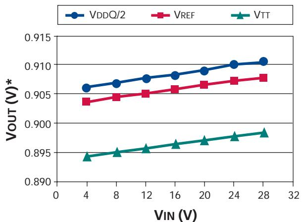
\* Test was performed with a 7A load on  $V_{DDQ}/2$  and a 0.3A load  $V_{TT}$
