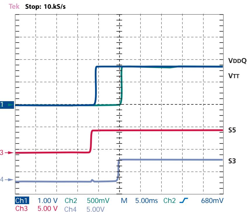
During an S3 state, the S3 control signal will go LOW and the system will enter a Suspend-to-RAM state (STR). STR can only occur after the DRAM has been properly placed into self refresh mode. This requires a predefined series of command sequences (turn off ODT, precharge all banks, synchronously take CKE LOW with the AUTO REFRESH command). Please see any Micron DDR2 data sheet for all requirements.
