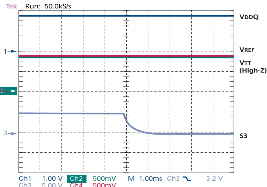
Note: During Suspend-to-RAM, all supply voltages must be maintained within specified data sheet values, including VREF. VTT is not required during STR.
