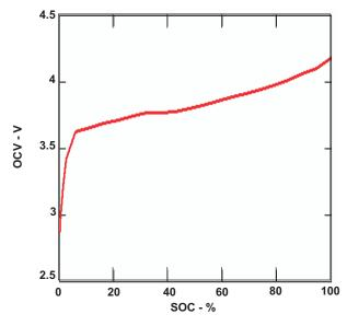
Figure 3. SOC Dependency on OCV
