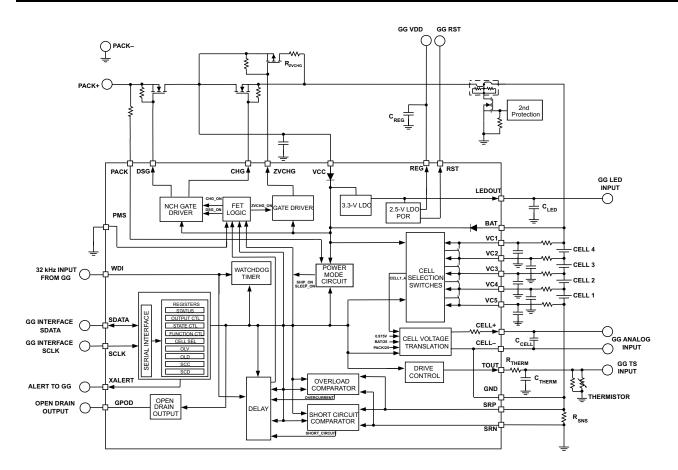
Figure 5. bq29330 Functional Block Diagram
