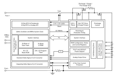
Figure 1. Battery Management Unit Block Diagram
