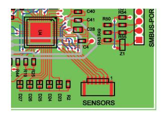
Figure 16. Layout of Temperature Sensor Signals
