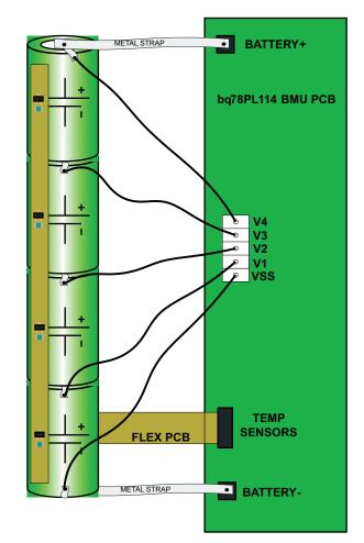
Figure 1. Battery to BMU Power, Cell Voltage, and Temperature Connections
