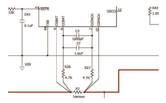
Figure 6. Current Measurement Circuit
