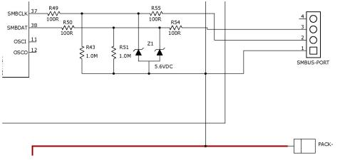
Figure 12. SMBus Interface Circuit
