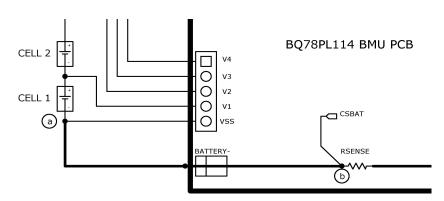
Figure 2. Battery–Connection Voltage Drop Requirements: V<sub>ab</sub> < 100 mV During Charge
