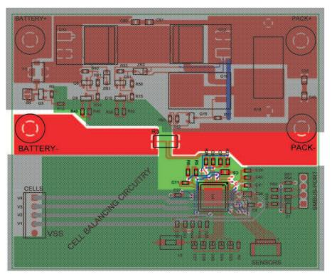
Figure 15. Layout of Current Sense Resistor and Sense Signal Lines (CCBAT, CCPACK, etc.)
