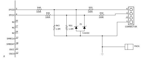
Figure 13. EFCIx Interface Circuit
