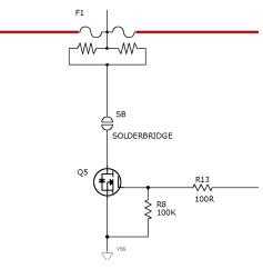
Figure 8. Chemical Fuse Circuit
