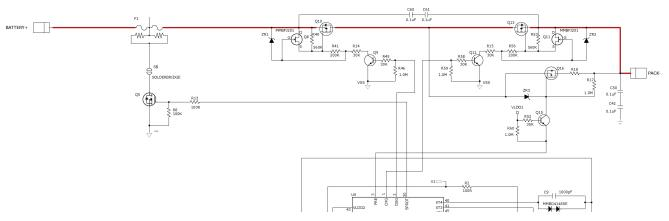
Figure 7. Pack Disconnect Switches
