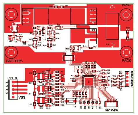
Figure 18. Top Layer of Finished Design
