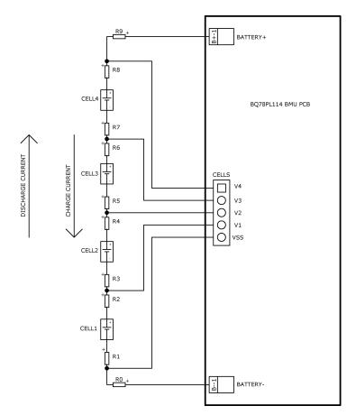
Figure 3. Schematic of Battery Sense Connections and System Impedances
