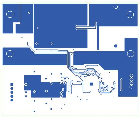
Figure 21. Bottom Layer of Finished Design
