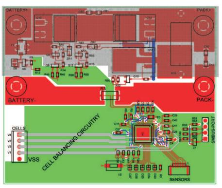
Figure 14. VSS Star Ground and Internal Copper Plane
