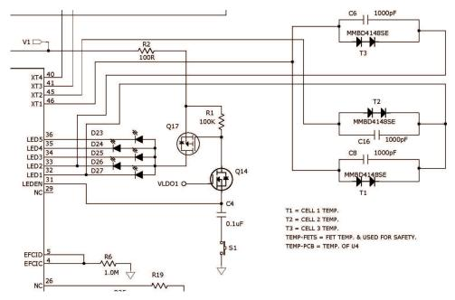
Figure 9. Pushbutton Circuit and LED SOCi Display for bq78PL114 With FW4452
