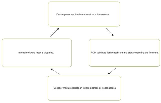
Figure 1. Reset Loop Mechanism
