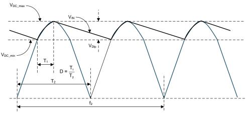
Figure 2. AC Rectified Waveform
