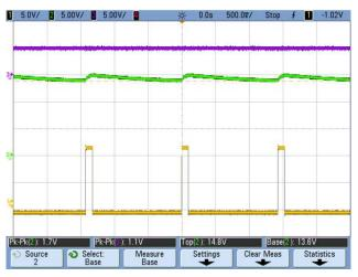
Figure 13. 90 VAC: No Load on 12-V Output, 5-V Load Transient
