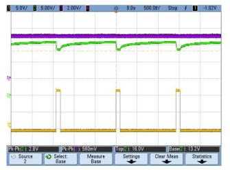
Figure 19. 90 VAC: Full Load on 5-V Output, 12-V Load Transient
