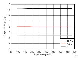
Figure 6. Full Load on 5 V and 5 mA on 12.5 V (Line Regulation)
