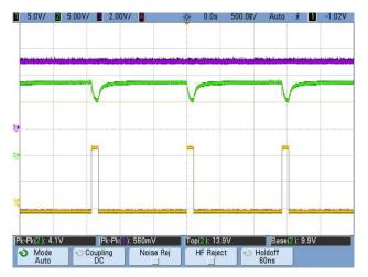
Figure 17. 90 VAC: No Load on 5-V Output, 12-V Load Transient
