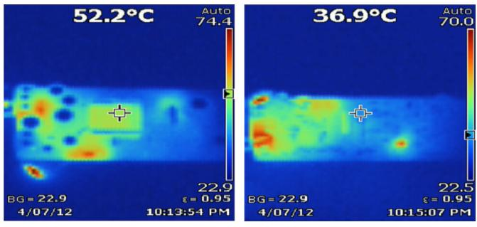
Figure 8. Thermal Performance: 240-VAC Full Load (Top)
