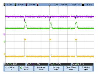
Figure 15. 90 VAC: Full Load on 12-V Output, 5-V Load Transient
