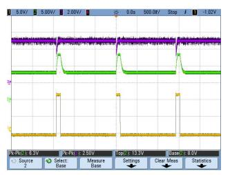
Figure 16. 480 VAC: Full Load on 12-V Output, 5-V Load Transient
