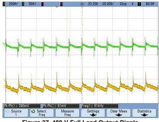
Figure 37. 480-V Full Load Output Ripple
