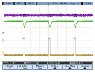
Figure 18. 480 VAC: No Load on 5-V Output, 12-V Load Transient
