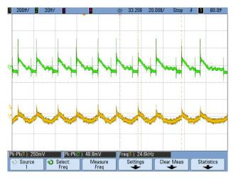
Figure 35. 90-V Full Load Output Ripple
