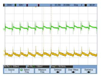
Figure 36. 230-V Full Load Output Ripple
