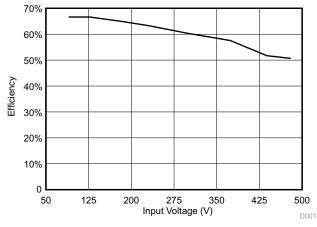
Figure 4. Full Load Efficiency vs Line Voltage
