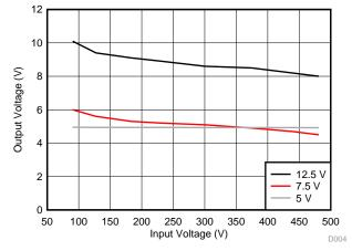
Figure 7. No Load on 5 V and 5 mA on 12.5 V (Line Regulation)
