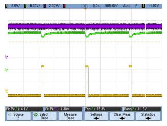
Figure 20. 480 VAC: Full Load at 5 V, 12-V Load Transient
