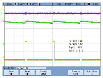
Figure 14. 480 VAC: No Load on 12 V, 5-V Load Transient
