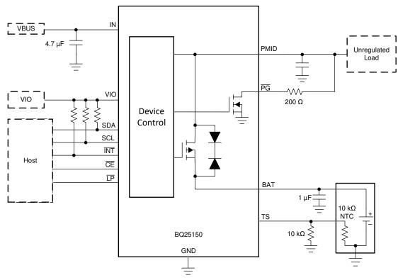
Figure 1. Discharge Schematic
