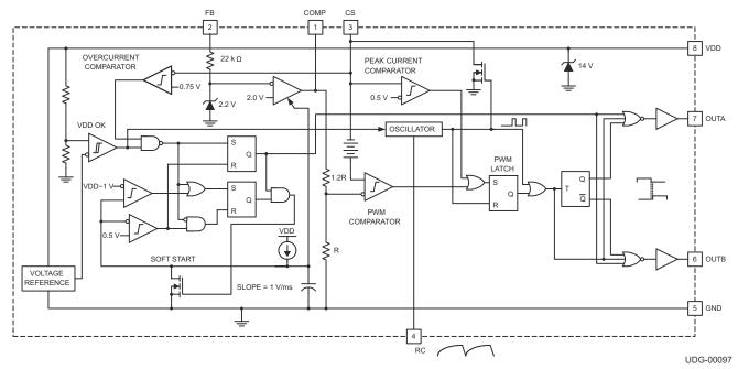
Figure 1-1. Functional Block Diagram
