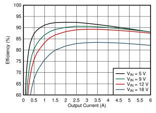
Figure 3-1. TPSM843620 Efficiency Graph
