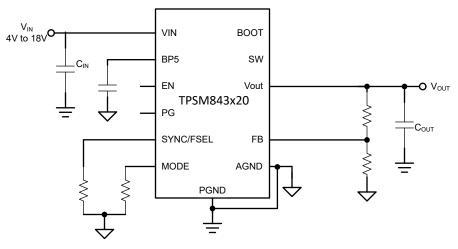
Figure 2-6. TPSM843620 Simplified Schematic
