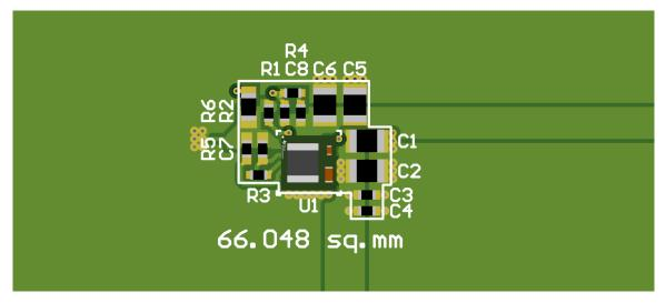
Figure 2-3. TPSM843620 PCB Design Size
