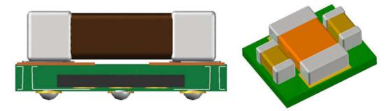
Figure 2-1. MicroSiP Package Example
