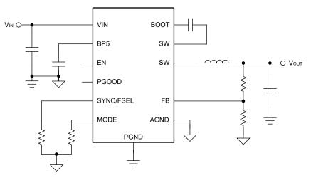
Figure 2-5. TPS543620 Simplified Schematic
