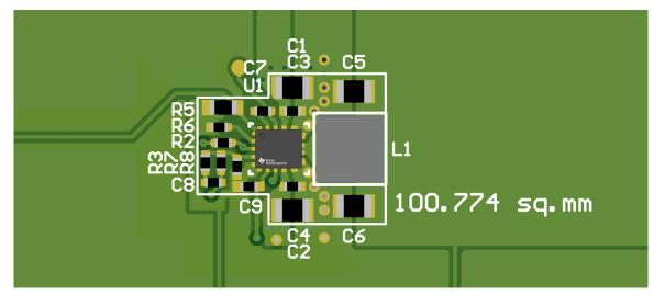
Figure 2-2. TPS543620 PCB Design Size
