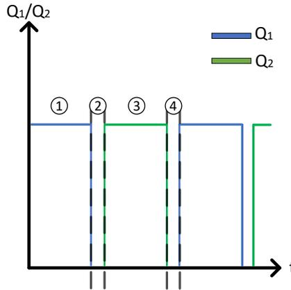
**Figure 3-1. Time Diagram of PWM Signal**
