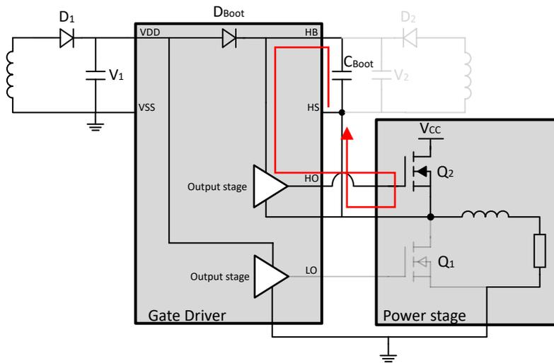
Figure 3-5. Equivalent Circuit in Mode 3
