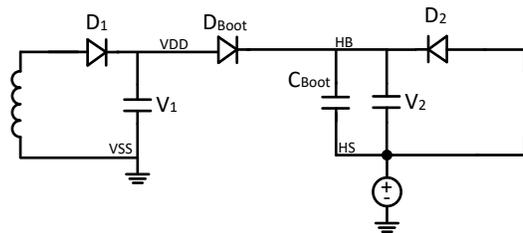
**Figure 3-9. Schematic With  $V_2$  Connected**
