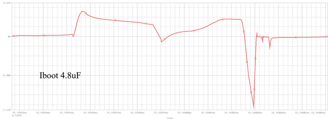
**Figure 3-11. Simulation Results (D=99.5% With 4.7uF Bootstrap Capacitor)**
