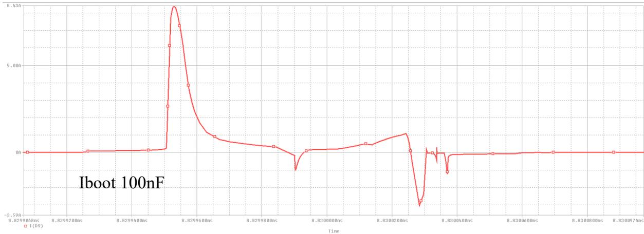
**Figure 3-10. Simulation Results (D=99.5% With 100nF Bootstrap Capacitor)**
