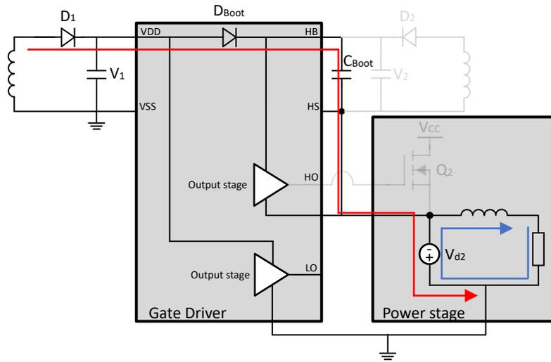
Figure 3-4. Equivalent Circuit in Mode 2
