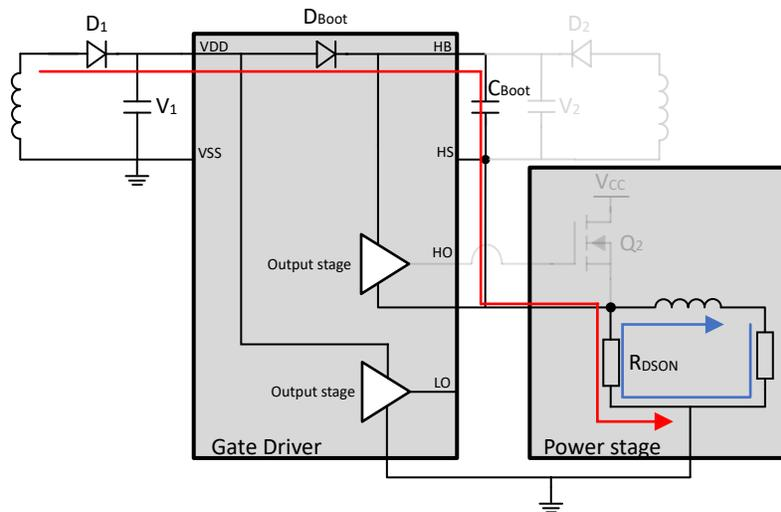
**Figure 3-3. Equivalent Circuit in Mode 1**
