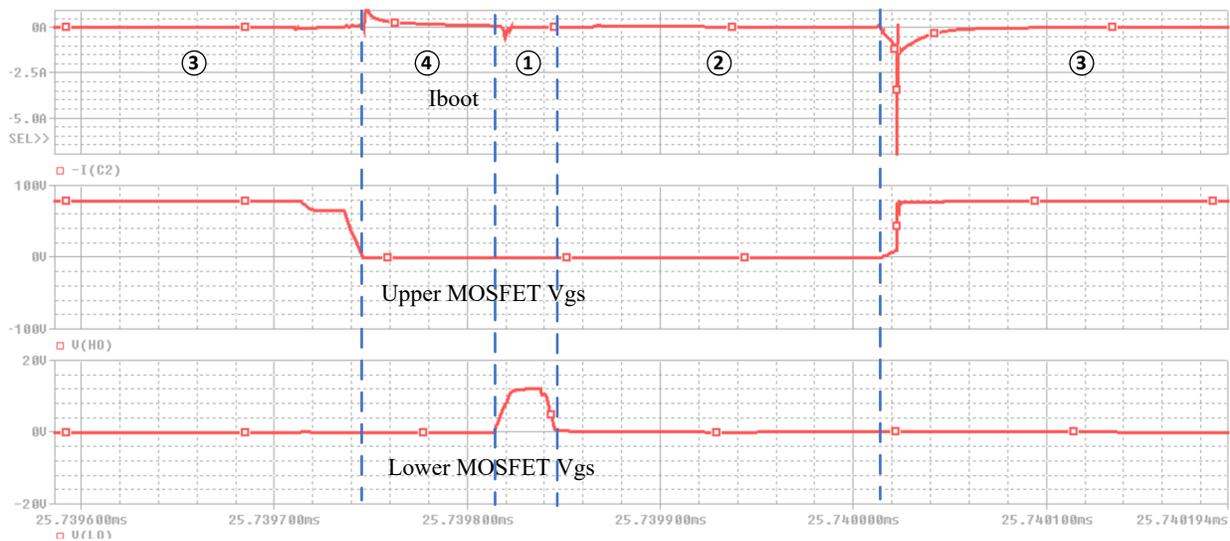
**Figure 3-8. Simulation Results (D=99% With Reverse Recovery Characteristic)**
