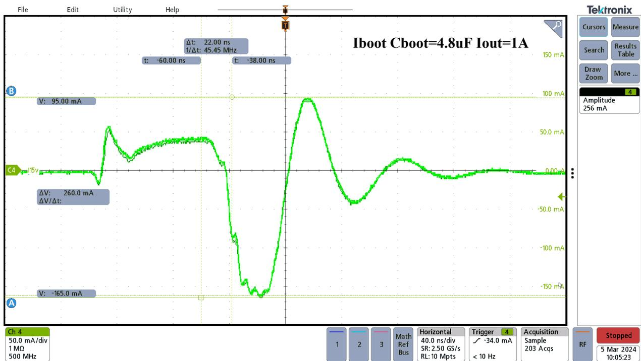
Figure 3-13. Experiment Results (4.8uF Bootstrap Capacitor)
