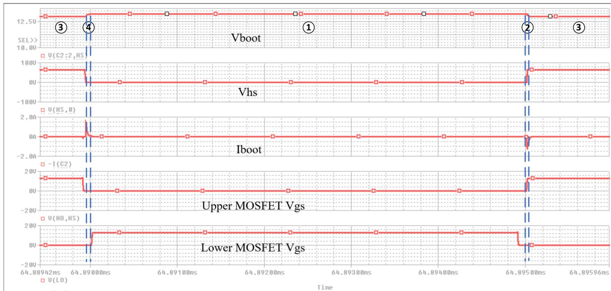
**Figure 3-6. Simulation Results (D=50%,  $C_{boot}$ =100nF)**
