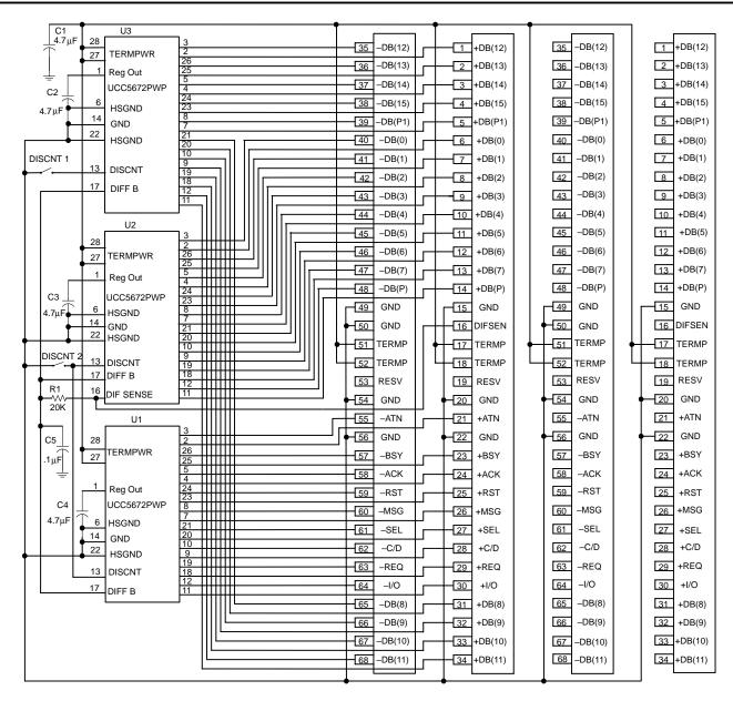
NOTE: Enlarge the ground area and use all heat sink pins to conduct heat away from the UCC5672.
