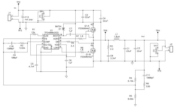
Figure 1. Application Diagram for the TPS40002/3
