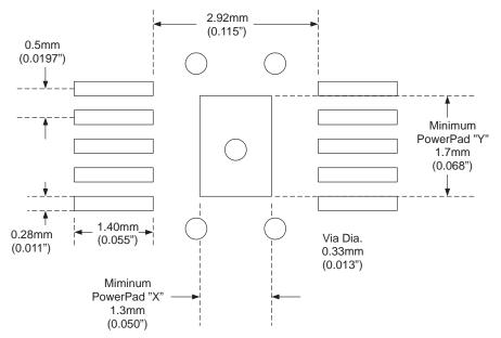
Figure 3. PowerPAD PCB footprint information
