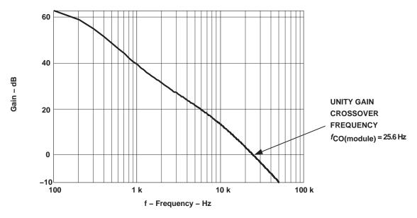
Figure 6. Power Module Bode Plot
