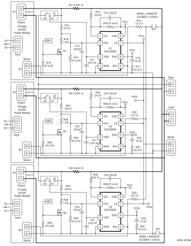
Figure 1. Three Module Load Share Application
