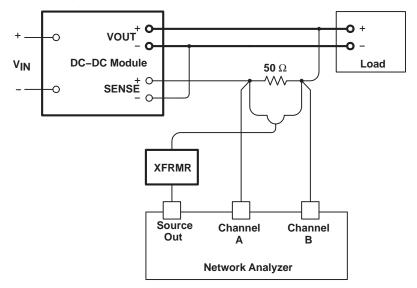
Figure 5. Measuring the Unity Gain Crossover Frequency
