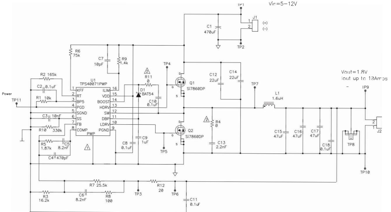
Figure 3-1. TPS40071EVM-001 Schematic
