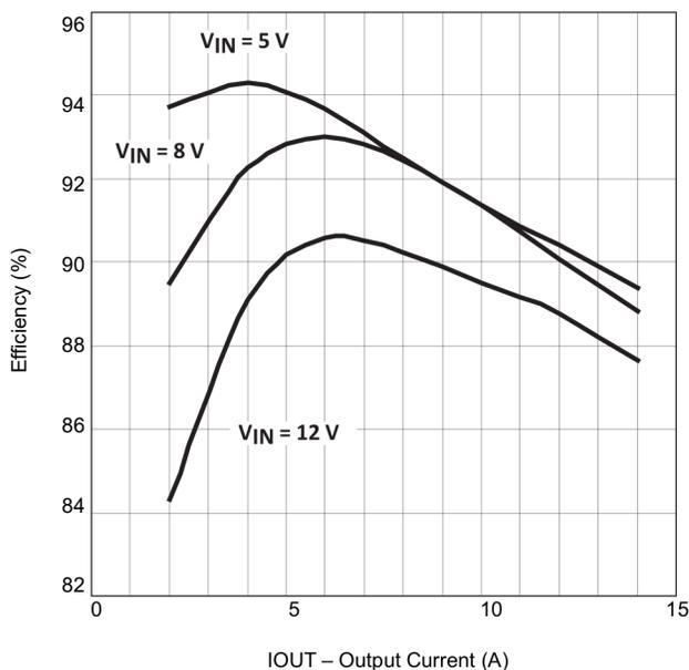
**Figure 5-2. Efficiency vs Output Current ( $V_{OUT} = 1.8\text{ V}$ )**
