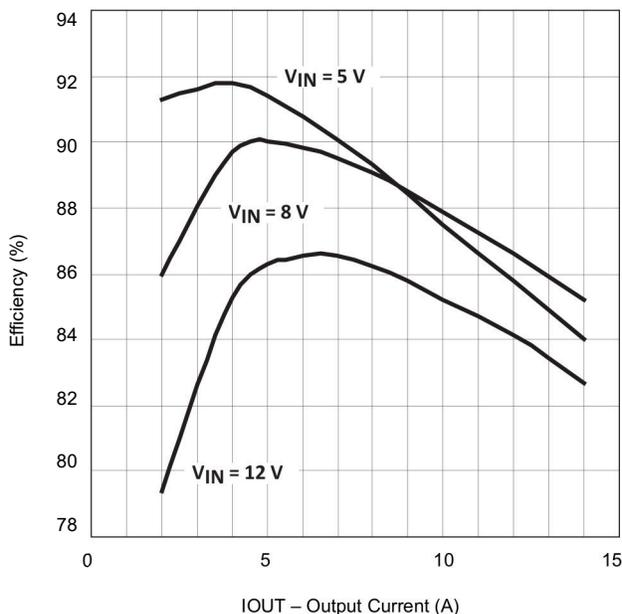
**Figure 5-1. Efficiency vs Output Current ( $V_{OUT} = 1.2\text{ V}$ )**
