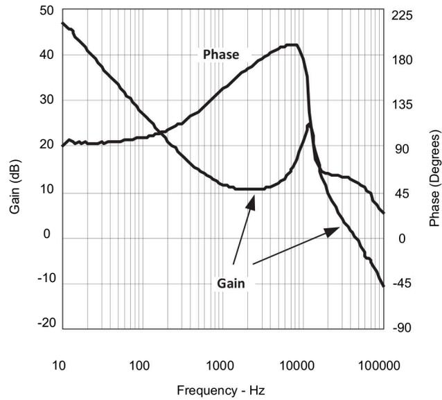
**Figure 5-5. Gain/Phase vs Frequency ( $V_{IN} = 5\text{ V}$ )**
