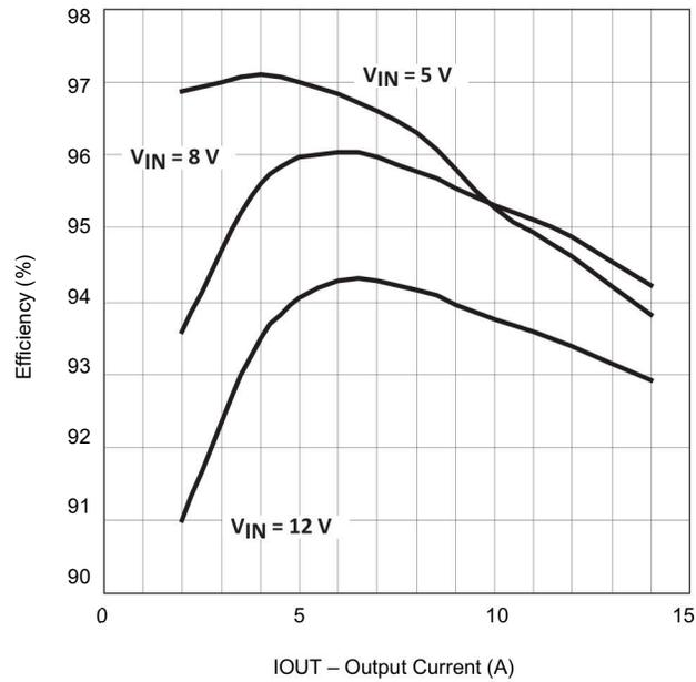
**Figure 5-3. Efficiency vs Output Current ( $V_{OUT} = 3.3\text{ V}$ )**
