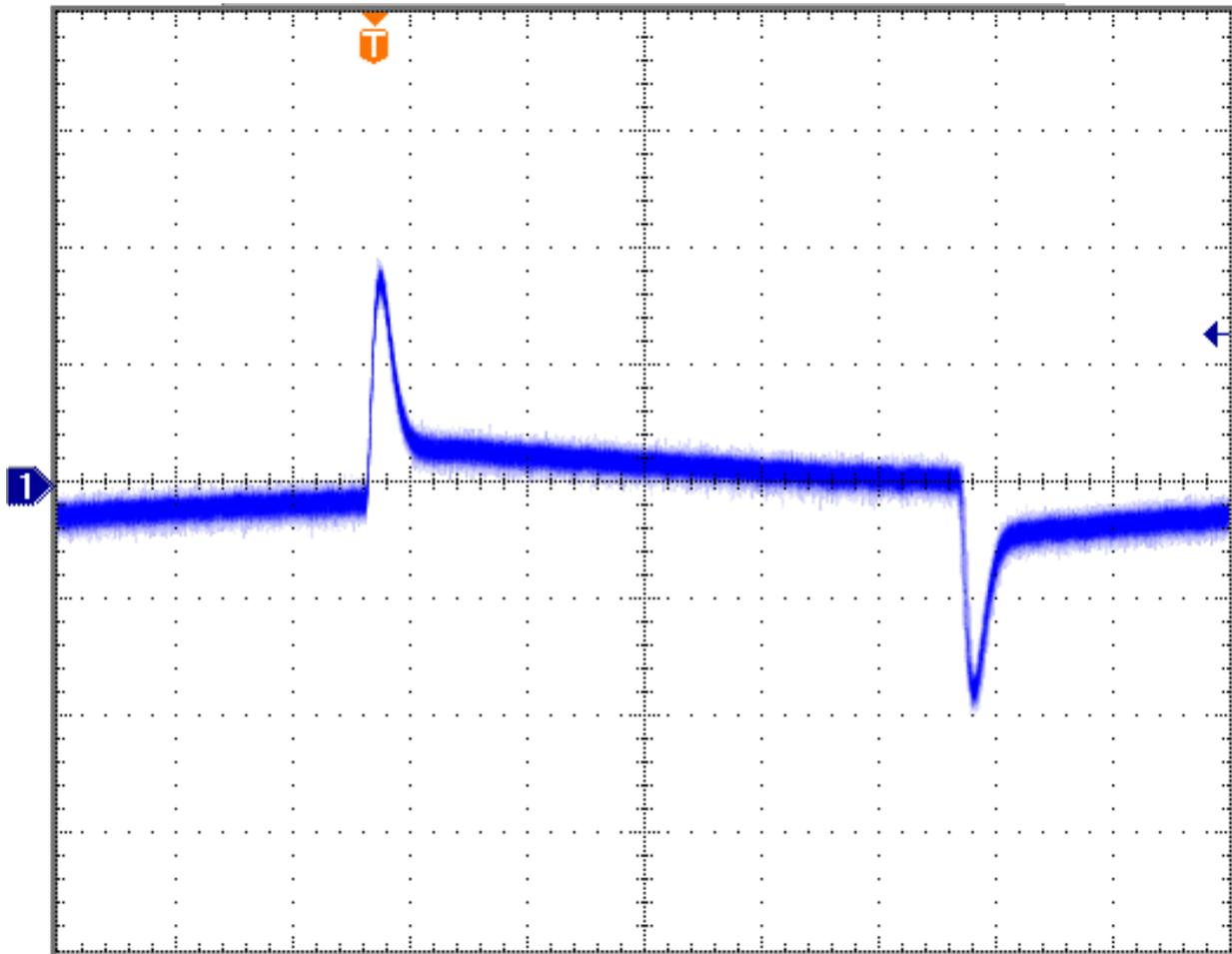
**Figure 5-4. Output Voltage with 5-A Load Step**
