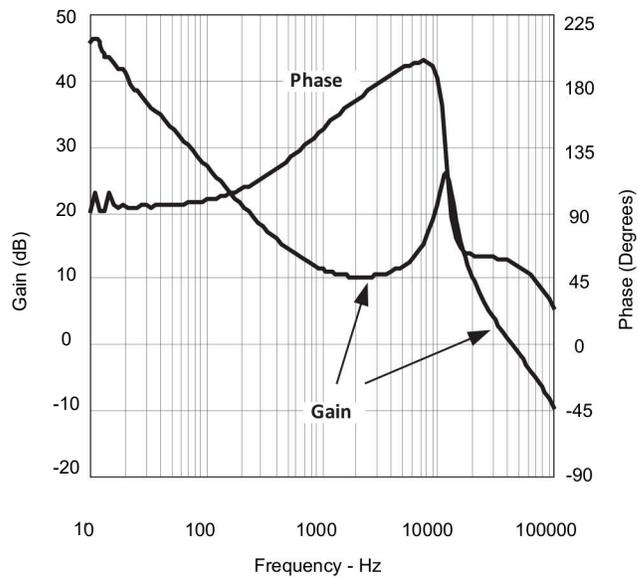
**Figure 5-6. Gain/Phase vs Frequency ( $V_{IN} = 12\text{ V}$ )**
