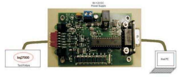
Figure 1. bq27x00 Test and Program Board
