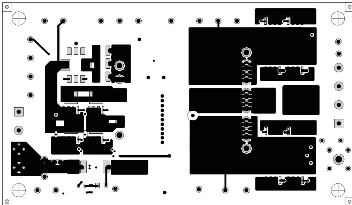
Figure 12. PCB Top Copper
