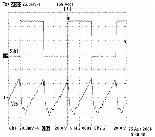
Figure 10. Top: Q3  $V_{DS}$ ; Bottom: CS Pin
