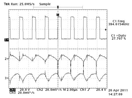
Figure 9. Switching-Node Waveform (CH1 = Phase (TP15), Ch2 = Vo1 ripple, Ch3 = Vo2 ripple,  $V_{\rm IN}$  = 48 V, lo1 = lo2 = 50 mA)
