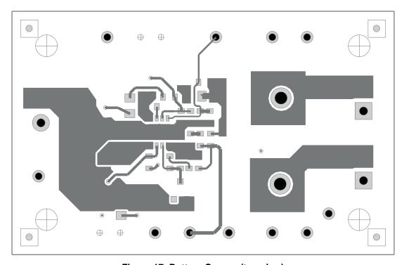
Figure 17. Bottom Copper (top view)
