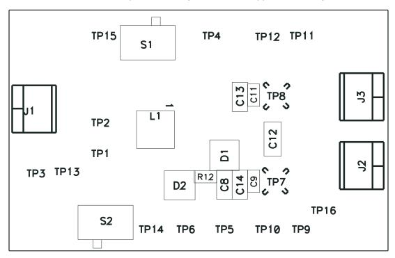
Figure 12. UCC25230EVM-754 Top Layer Assembly Drawing (top view)
