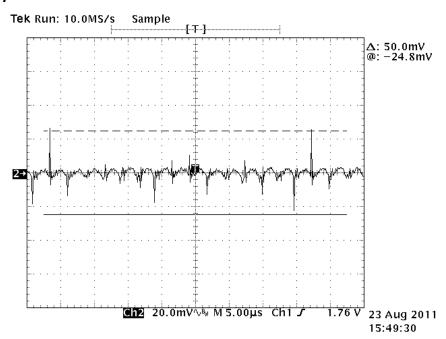
Figure 8. Output Ripple  $(V_{IN} = 48 \text{ V}, Io1 = Io2 = 50 \text{ mA from Vo1 (TP8) or Vo2 (TP7)})$
