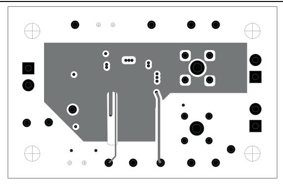
Figure 16. Internal Layer 2 (top view)
