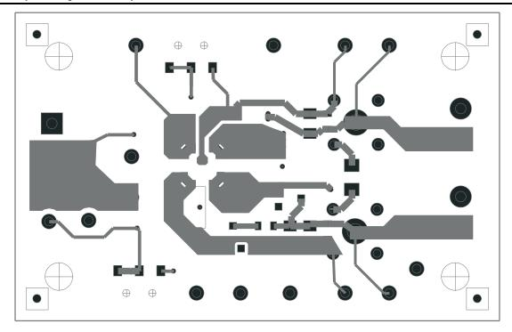
Figure 14. Top Copper (top View)
