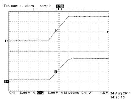
Figure 10. Enable Turn-On Waveform  $(V_{IN} = 48 \text{ V}, Io1 = Io2 = 50 \text{ mA}, Ch1: Vo1 (TP8), Vo2 (TP7))$
