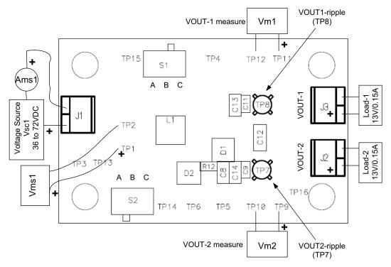
Figure 2. UCC25230EVM-754 Recommended Test Set Up
