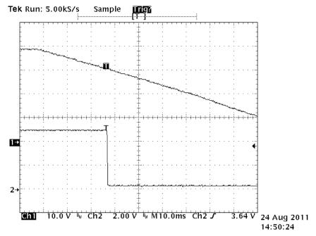
Figure 11. Enable Turn-Off Waveform (lo1 = lo2 = 50 mA, Ch1:  $V_{\rm IN}$  (TP1, 2), Ch2: VIN\_G (TP4))
