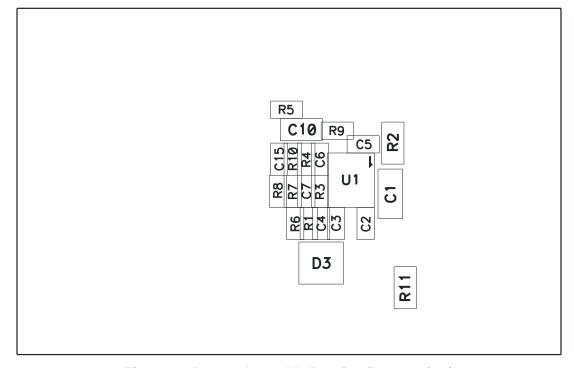
Figure 13. Bottom Assembly Drawing (bottom view)
