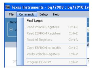
Figure 6. Commands Without Communication Established
