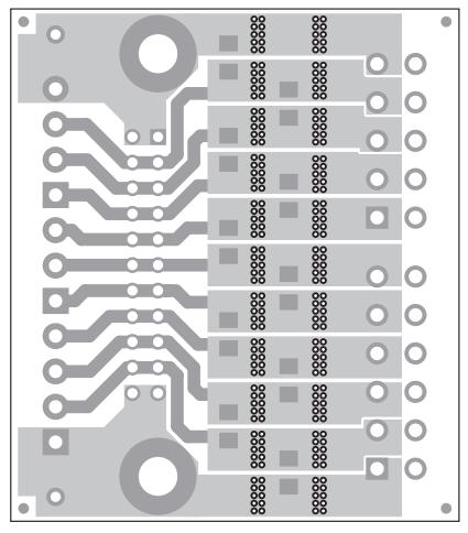
Figure 21. Resistor Simulator Top Layer
