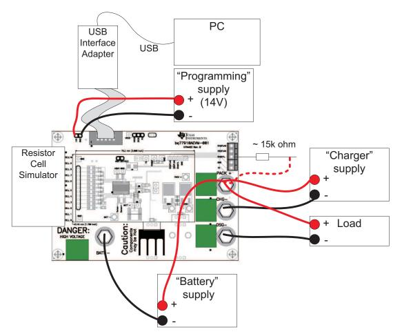
Figure 3. EVM Connection for Communication and Programming
