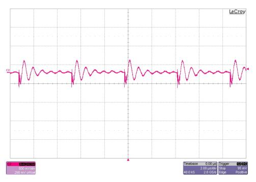
The 26.2V output ripple voltage is shown in the figure below. The image was taken with the output loaded to 6A and the input voltage set to 26Vdc. (500mV/DIV, 2us/DIV)
