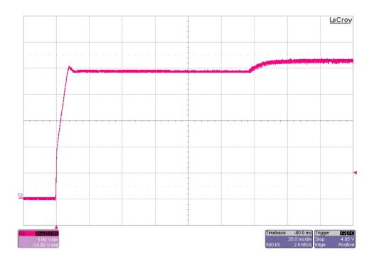
The figure below shows the 26.2V output voltage startup waveform after an input voltage of 25V is applied. Iout = 10A. (5V/DIV, 20ms/DIV)
