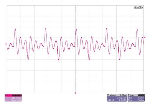
The 26.2V output ripple voltage is shown in the figure below. The image was taken with the output loaded to 6A and the input voltage set to 12Vdc. (500mV/DIV, 2us/DIV)
