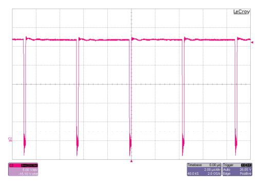
The photo below is of the FET switch node voltage at TP7. The input voltage is 26Vand the output is loaded to 1A. (5V/DIV, 2us/DIV)
