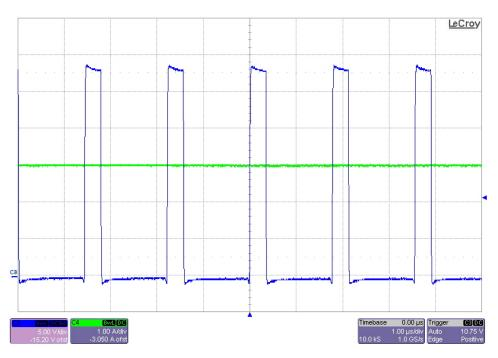
The photo below is of the FET switch node voltage at TP19. The input voltage is 28Vand the output cap bank voltage is at 15V while being charged at 3A. A 28.2F/29.7V cap bank was used. (5V/DIV, 1A/DIV, 1us/DIV)
