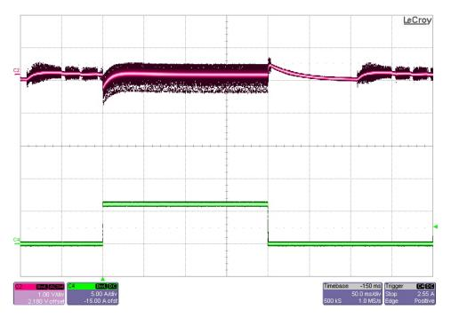
The photo below shows the 26.2V output voltage (AC coupled) when the load current is switched between 0A and 10A. Vin= 20V (1V/DIV, 5A/DIV, 50ms/DIV)
