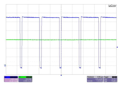
The photo below is of the FET switch node voltage at TP19. The input voltage is 28Vand the output cap bank voltage is being regulated at 25.2V (charge current reduced). A 28.2F/29.7V cap bank was used. (5V/DIV, 1A/DIV, 1us/DIV)
