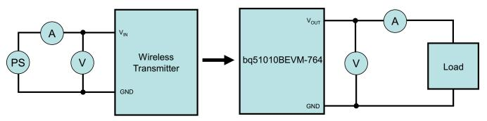
Figure 2. Test Set Up
