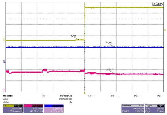
Figure 3. Load Step, 0 mA to 600 mA
