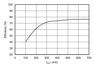
Figure 6. Efficiency for the bq51010B versus I<sub>out</sub>
