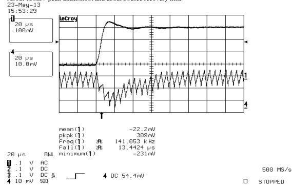
Load dump response: 48Vin and DC load of 6A off the 30Vout; additional 6A removed at about -1A per usec: Top trace (scope channel 4 with external Tektronix current probe) is load current at 2A per division; bottom trace (scope channel 1) is Vout
