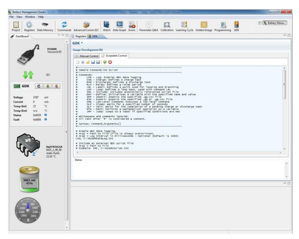
Figure 7. GDK Plug-in—Scriptable Control Tab
