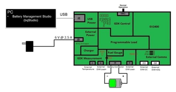
Figure 9. GDK Optional Configuration—Onboard Fuel Gauge
