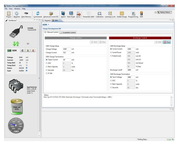
Figure 6. Manual Control Tab—Discharge Control Panel While Discharging
