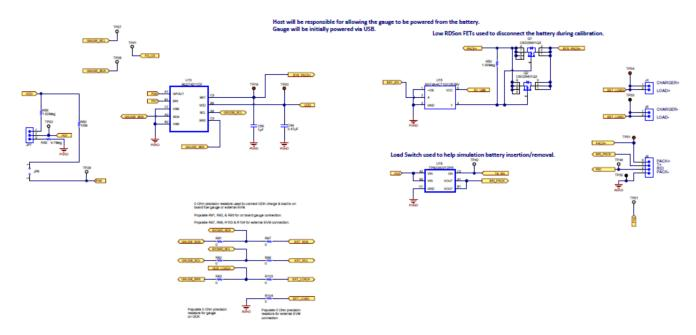
Figure 17. GDK Schematic—Battery Connection and Fuel Gauge
