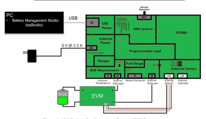
Figure 8. GDK Default Configuration—External EVM Connected
