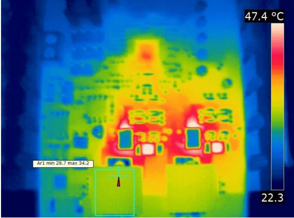
PMP8999B 12.00Vin 2.948Ain 1.0120Vout 30.0A no fan >20 minutes ambient 22 degrees Celsius 351kHz per phase Snubbers hottest at 73deg. C; area near Q3 max 71; near Q4 68.5; inductor tops 58 and 56; controller 61
