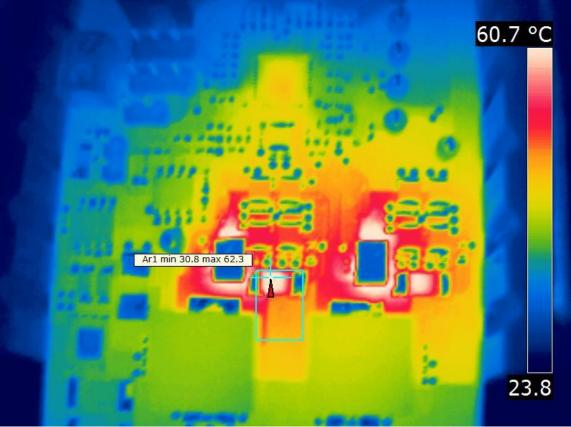
12.18Vin 2901mA in 30.07Aout 1.0077Vout same 351kHz per phase IR2863 with 51 max PMP8999B model t2 with drive updates 12.2Vin 1Vout at 30.1A 351kHz / phase 12.0V fan 6.5" from board ambient at 23 deg. C Hottest PCB near Q3 at 49; near Q4 at 47.5 choke tops at 36 & 34; snubbers 50 & 51
