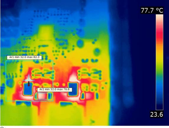
12.21Vin 3.939Ain 40.08Aout 1.0089 at TPs or 7.658W loss IR2862 with 66-67 max PMP8999B model t2 with drive updates 12.2Vin 1Vout at 40.1A 351kHz / phase 12.0V fan 6.5" from board ambient at 23 deg. C Hottest PCB near Q3 at 67; near Q4 at 63 choke tops at 43 & 41; snubbers 61 & 62
