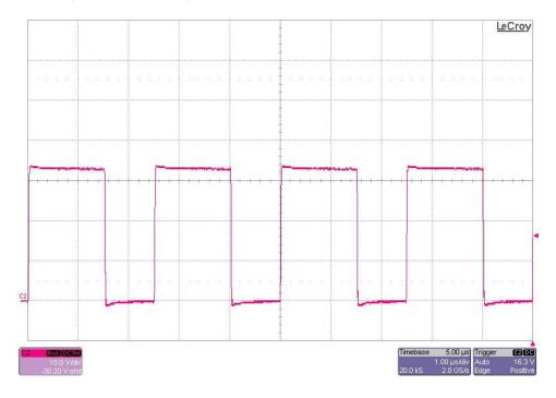
The photo below is the switch-node waveform (TP5). The input voltage is 27V and the output is loaded to 3A. (10V/DIV, 1uS/DIV)
