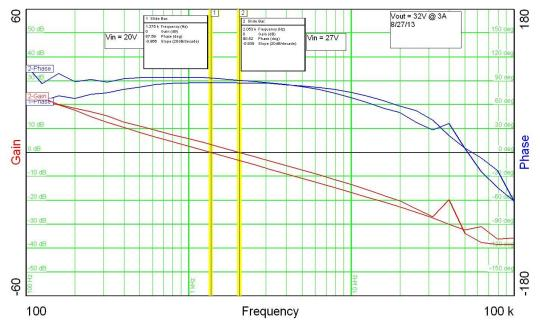
The plot below shows the loop gain with the input voltage set to 20V and 27V and the output loaded to 1A.
