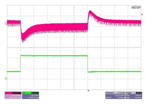
The photo below shows the 32V output voltage (AC coupled) when the load current is stepped from 1.5A to 3A (50% - 100%). Vin = 24Vdc (200mV/DIV, 1A/DIV, 2mS/DIV)
