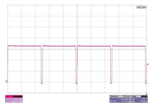
The photo below is the switch-node waveform (TP5). The input voltage is 20V and the output is loaded to 0.51A. The converter operates in CCM above this current level. (10V/DIV, 1uS/DIV)
