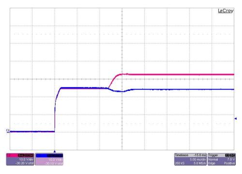
The photo below shows the 32V output voltage startup waveforms after the application of 24Vdc in. The output was loaded to 3A. (10V/DIV, 5mS/DIV)
