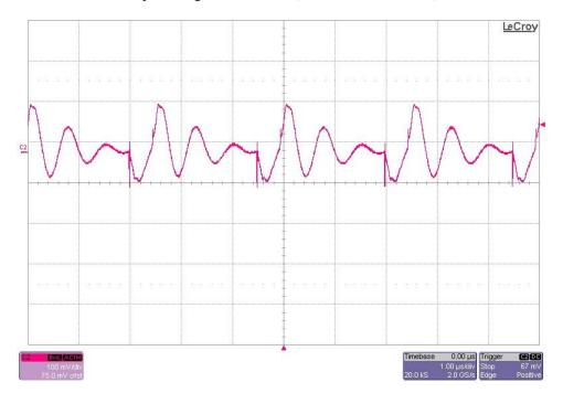
The 32V output ripple voltage (AC coupled) is shown in the figure below. The image was taken with the output loaded to 3A and the input voltage set to 24Vdc. (100mV/DIV, 1uS/DIV)
