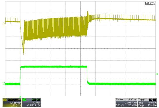
8.4 10mA to 1.5A Transient – 230VAC/50Hz Input
