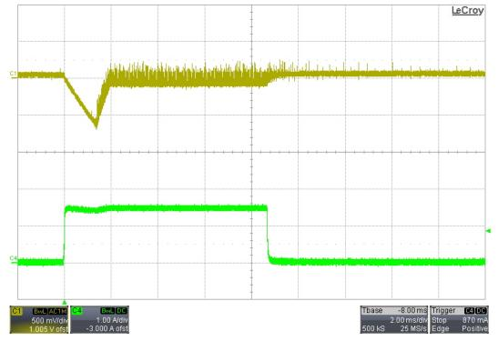
8.2 0A to 1.5A Transient – 230VAC/50Hz Input
