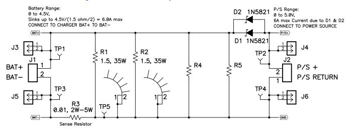
Figure 2. BAT Load (PR1010) Schematic
