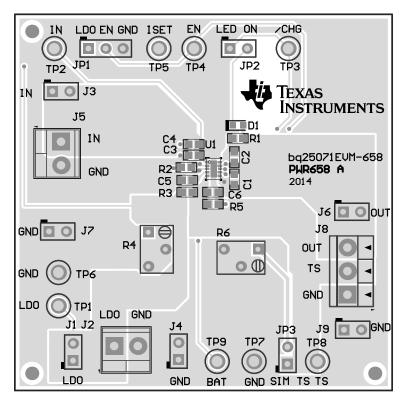
Figure 3. Top Assembly Layer
